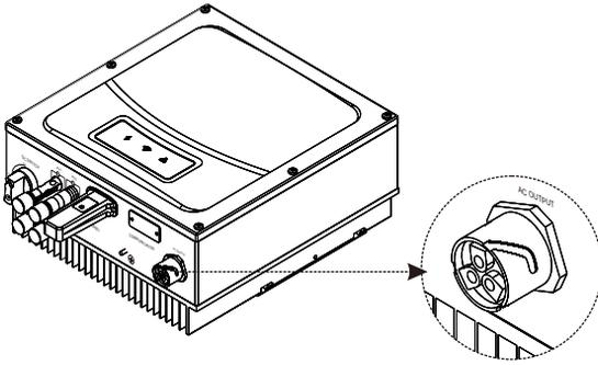
2. Remove the parts of the AC connection plug from the accessory bag. Prepare the pressure screw, sealing ring, threaded sleeve over the AC cable
