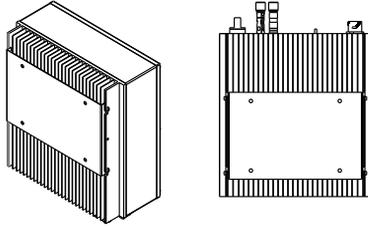
2. Hook the inverter to the rear panel. Using an M5 screw to secure the inverter to the mounting frame to ensure safety.
