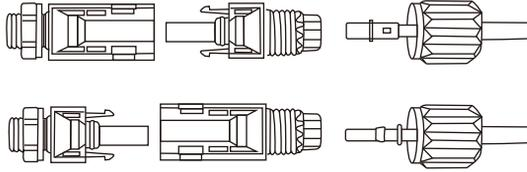
**Step 5** Insert the positive and negative connectors into corresponding DC input terminals of the PH5000 until you hear a "click" sound.
