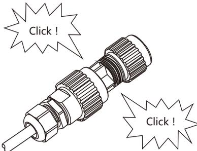
5. Finally, insert the AC connection plug into the AC connection receptacle on the inverter.
