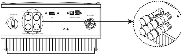
The diagram drawing of DC side is shown as below, notice that the connectors are in paired (male and female connectors). The connectors for PV arrays and inverters are H4 (yunfan) connectors;
