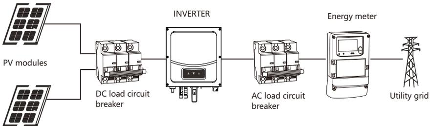
The inverter may only be operated with a permanent connection to the public power grid. The inverter is not intended for mobile use. Any other or additional use is not considered the intended use. The manufacturer/supplier is not liable for damage caused by such unintended use. Damage caused by such unintended use is at the sole risk of the operator.
