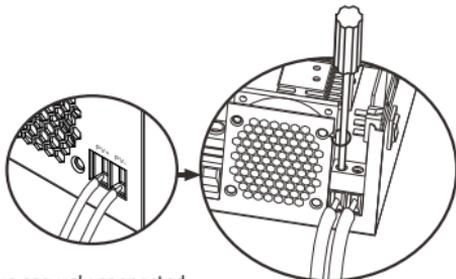
3. Make sure the wires are securely connected.
