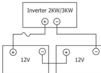
3. Insert the ring terminal of battery cable flatly into battery connector of inverter and make sure the bolts are tightened with torque of 2-3 Nm. Make sure polarity at both the battery and the inverter/charge is correctly connected and ring terminals are tightly screwed to the battery terminals.
